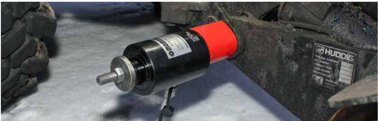
ACHC302 used here for removing shaft in back hoe loader.
